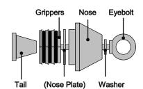
It is operated by simply inserting it into the pipe and turning the eyebolt. The turning action draws a cone into four toothed segments which are forced into the wall of the pipe. The harder the eye is pulled the harder the pipe is gripped. The grip is so good that it is possible to stretch the pipe!
